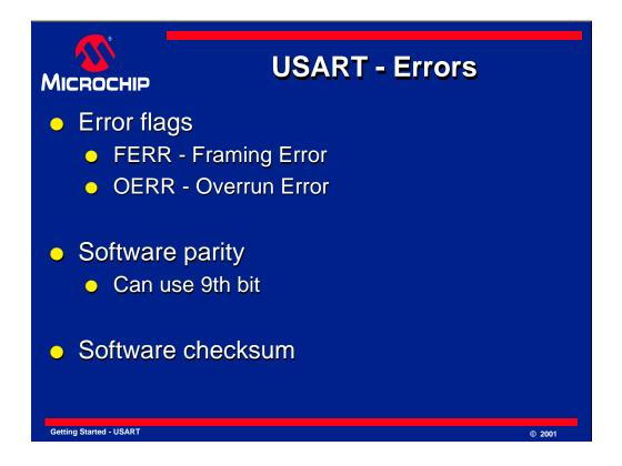
There are several errors that can occur during serial communications and the USART can detect two types of errors automatically. These are indicated by two error flags in the RCSTA register for framing errors and overrun errors.
